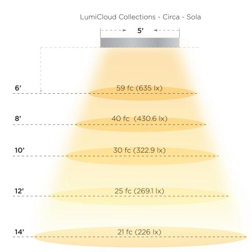
Note: Results are simulated based on 10'  $\times$  16' room & Reflection factors C70% W77% & F20% , other measurements available on requests.
